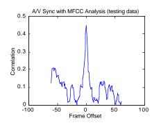
Figure 4: Correlation of audio and video data as the audio data is shifted in time past the video. (29.97 frames/sec.)
