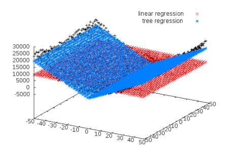
The red scatter plot shows the fit created by linear regression. The tree based regression fits two separate planes to the data that are shown as the blue scatter plot. The original noisy data is shown as the black dots.
