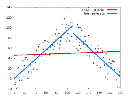
The blue line shows the result returned by tree regression and the red line the result of linear regression. • The result shown in the previous slide was obtained with the "jacobian\_choice=0" option for the Jacobian. As the reader will recall from the previous section, this option means that we did not use the refinement. When we turn on the option "jacobian\_choice=1" for refining the coefficients, we get the result shown below:
