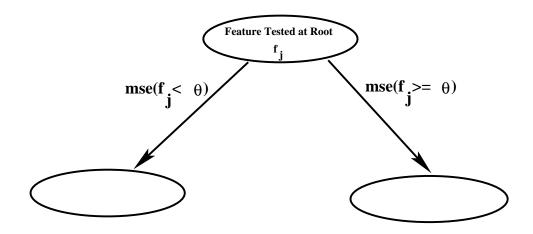
For each feature, you calculate the MSE (Mean Squared Error) per sample for every possible partition along the feature axis.
